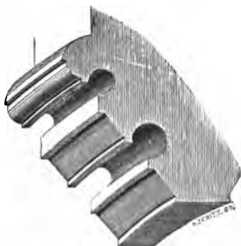
133. Finedon, Northamptonshire, c. 1340. The sunk chamfer and the hollow.
